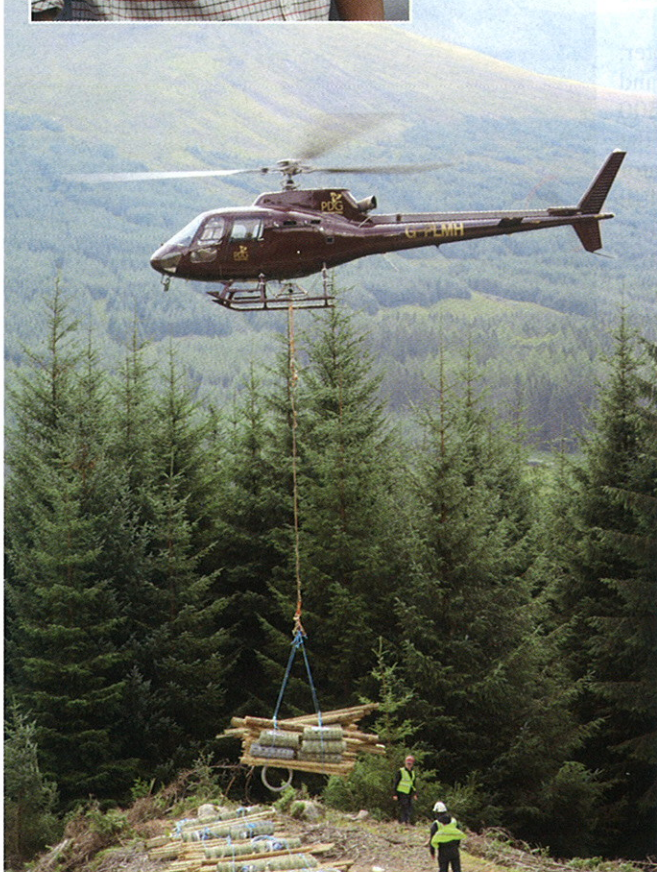
The helicopter is costly but efficient in areas where access by conventional vehicles would be difficult or impossible.
